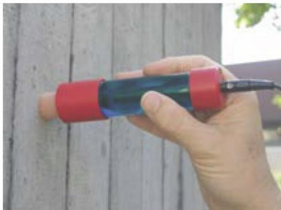
Standard half cell rod electrode
