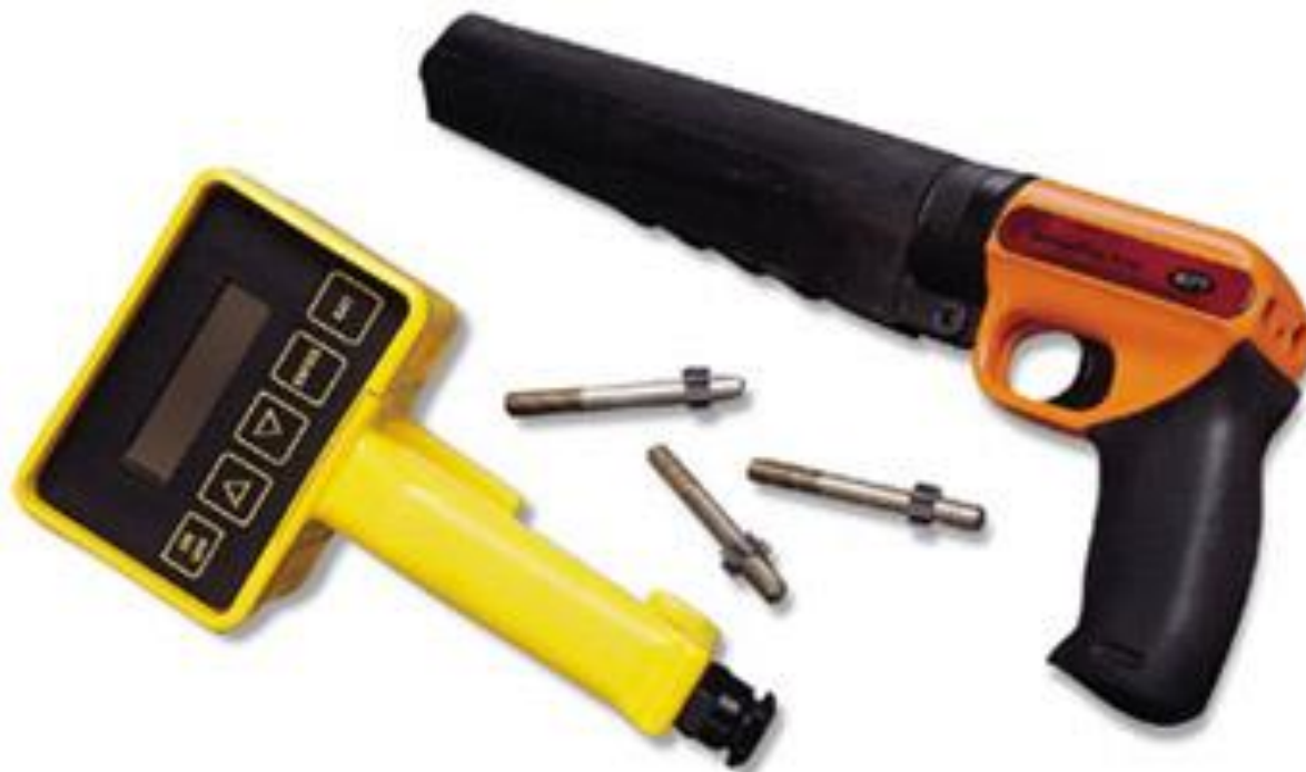
Windsor HP Probe - ASTM C-803
